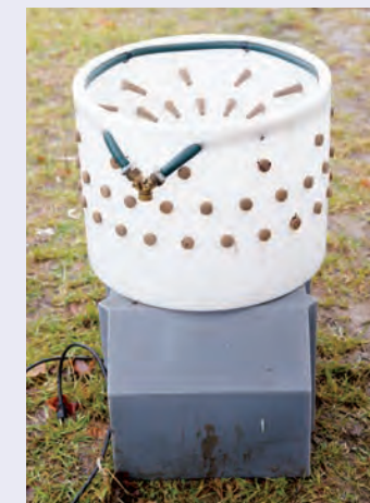
Deceptively simple in appearance, tub pluckers quickly turn a feathered bird into a clean carcass.
