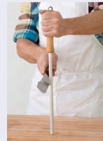
The frequent use of a honing rod is one of the keys to maintaining knife sharpness.
